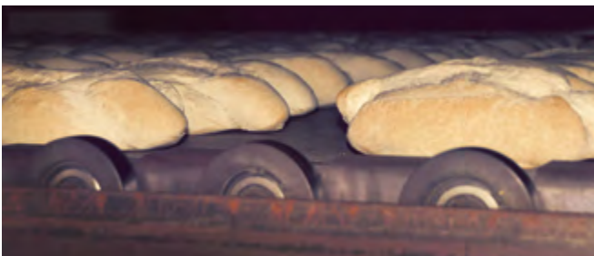
Baking oven chain with flanged roller and high temperature bearing (>600 F).
